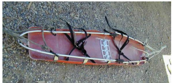
right railing brackets at the nose were pulled from the shell and one end of the litter railing sheared from the FastLock™ System. It was observed that the litter was still in one piece and could be considered functional although patient integrity could have been compromised. It was also observed that the railing of the litter was the cause of central failure due to buckling.
