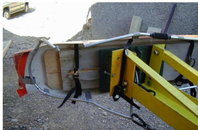
the bracket closest to the carabiner. At this point, the litter, while badly damaged was still attached to the litter harness by three of four attachment points. After several more seconds it was determined the litter had sustained enough damage to render it inoperable. Absolutely no damage was done to the <sup>1</sup>Fastlock™ System and the remnants of the litter were disassembled at the completion of the test.
