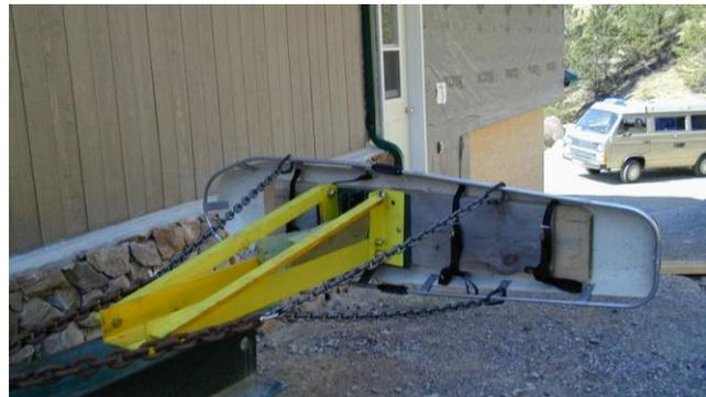
A rigid backboard was manufactured to place in the bottom of the litter to distribute the load of the SPD across the length of the litter. The footprint of the backboard was 60 inches by 11.25 inches. The distance from the center of the ram to the end of the litter was 47.25 inches and from the head of the litter to the ram was 34.75 inches.
